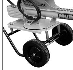
Place **Part F** Base Plate on **Part B** MudMixer Frame oriented as shown in the photograph (PIVOT LOCK RELEASE positioned on handle side) Secure Base Plate to Frame using Riser tubes (4) and 3/8" x 8" Bolts, Washers, Nuts. This replaces **Part J** hardware. You will not need the remaining 4 **Part J** hardware.
