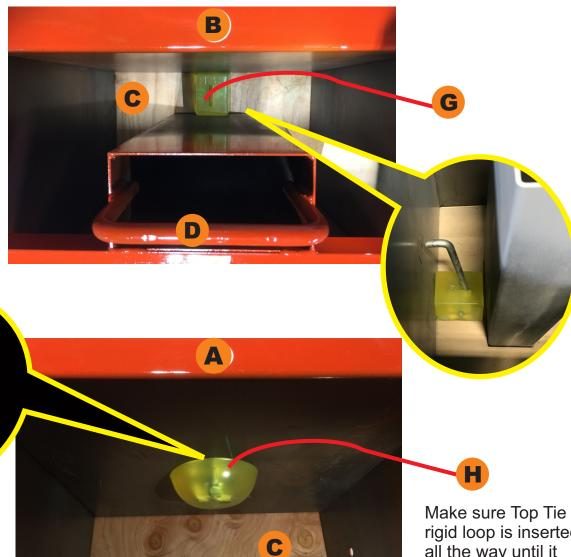
Make sure Top Tie off rigid loop is inserted all the way until it touches the metal. Keep slots clear of
