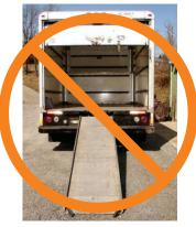
Carts with Blocks are not recommended up or down truck ramps or any steep ramps
