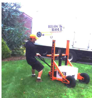
For best results pull block using black steering handle. For steep inclines a second person can push on the block from behind.
