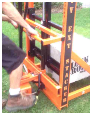
Pump right pedal until block is a few inches off the ground. (NEVER MOVE A BLOCK MORE THAN 6" OF THE GROUND)
