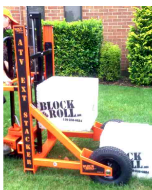
To stack 2 blocks, set up block to be raised behind the other block. Raise block using right pedal to clearance height, then push ATV EXT cart using orange push bar over other block. Use left pedal to lower.
