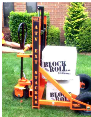
To stack 2 blocks, set up block to be raised behind the other block. Raise block using right pedal to clearance height, then push ATV EXT cart using orange push bar over other block. Use left pedal to lower.
