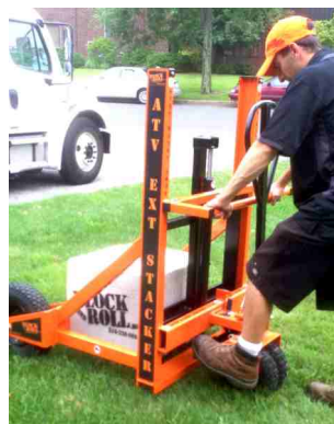
To lower block use pedal on the left. Adjust pressure from your foot to lower slow or fast.
